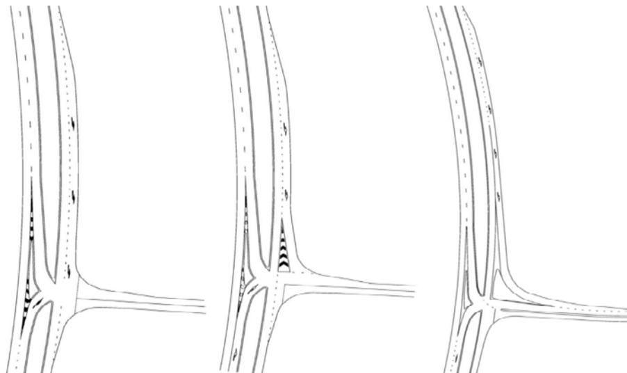
**Figure 3.1** Seagull Intersection at the Junction of Princes Highway and Island Point Road (left to right: 1996 installation, 2004 revision, 2007 revision) (Harper et al. 2011)
