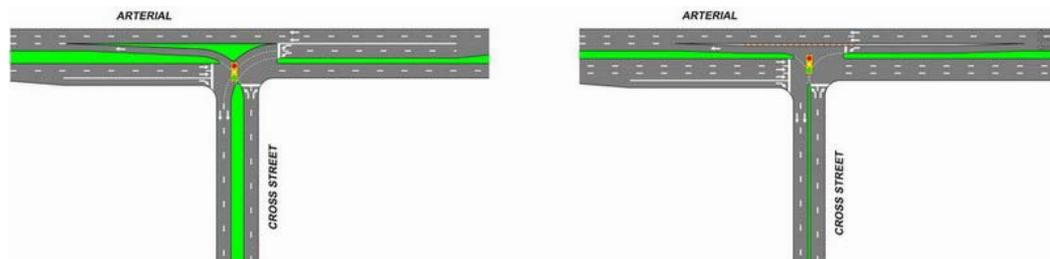
**Figure 1.4** Channelized (Merge-control) and Non-channelized (Lane-control) Seagull Intersections used in some parts of the United States (Office of Traffic, Safety & Operations 2007)
